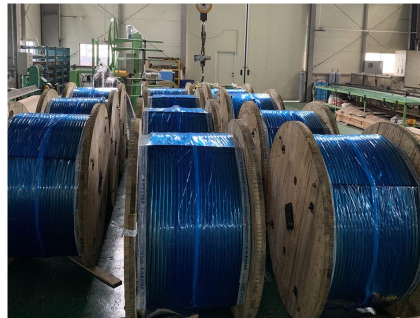
▲ S32750 Orbital-Welded Coil Tubing for umbilical manufacturing
